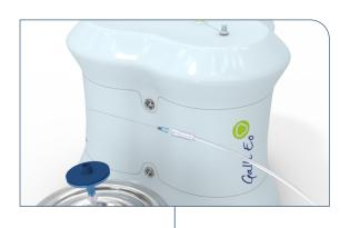
Connect the male luer of the outlet line of the generator to a sterile elution needle (size 21G-23G).
